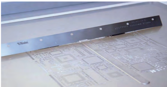
Figure 13: 3-D electroform stencil with notched e-blade.
