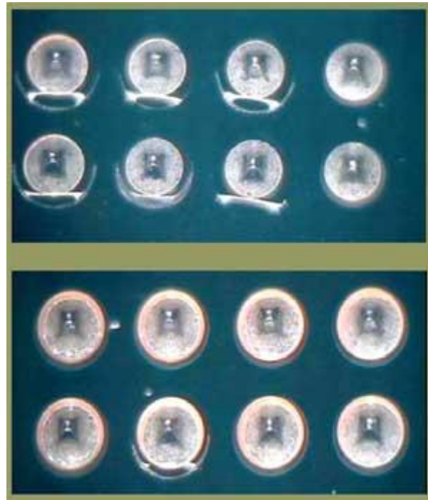
Figures 2A. Alt. header with small annular ring and B. with large annular ring, both 6-mil stencil.
