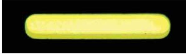
*[Figure 1a. Aperture side-wall smoothness of electroformed stencil.](#)*
