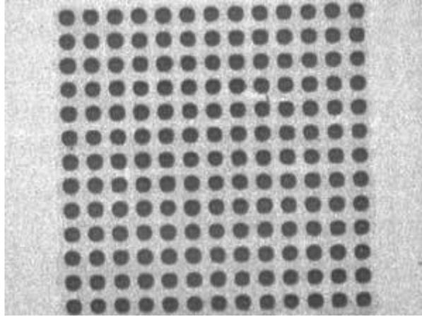
[Figure 2a. Solder bricks on 2<sup>nd</sup> print for 220-µm aperture for electroformed stencil using lead-free paste.](#)
