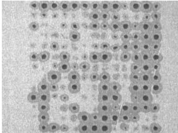
*Paste transfer from small apertures for tin/lead and lead-free* - Figures 2a/b show solder bricks printed on the second print cycle for both stencils using tin/lead and lead-free solder pastes for two different aperture sizes: 120-µm square and 220-µm square (shown). Several observations were made:
