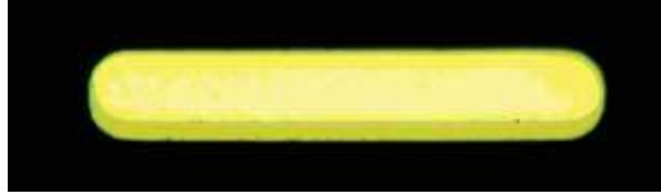
Figure 1a. Aperture side-wall smoothness of electroformed stencil.
