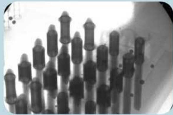
Figure 3A. On 93-mil-thick board: 6-mil stencil.
